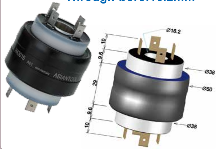
H43016 4poles/30A/AC250V Through-bore:16.2mm
